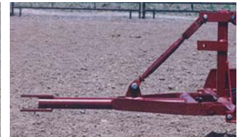
Tongue and Screwjack for pulling without a 3-point hitch
